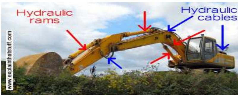
Photo: There are several different hydraulic rams at work in this digger. The rams are shown by red arrows and the narrow, flexible hydraulic pipes and cables that feed them in blue.
