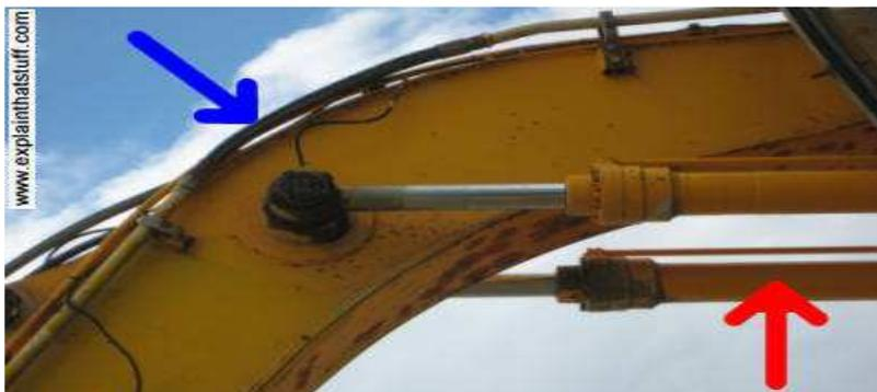
Photo: Close-up of a digger's hydraulic rams.
