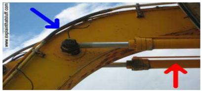
Photo: Close-up of a digger's hydraulic rams.
