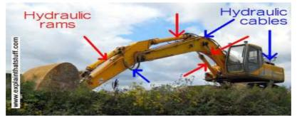
Photo: There are several different hydraulic rams at work in this digger. The rams are shown by red arrows and the narrow, flexible hydraulic pipes and cables that feed them in blue.
